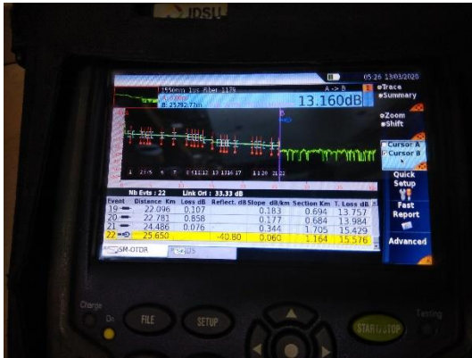
Mumbai Surat Span I OTDR Readings
