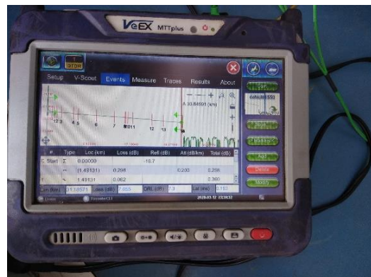
Umargaon - Dahanu Span OTDR Reading
